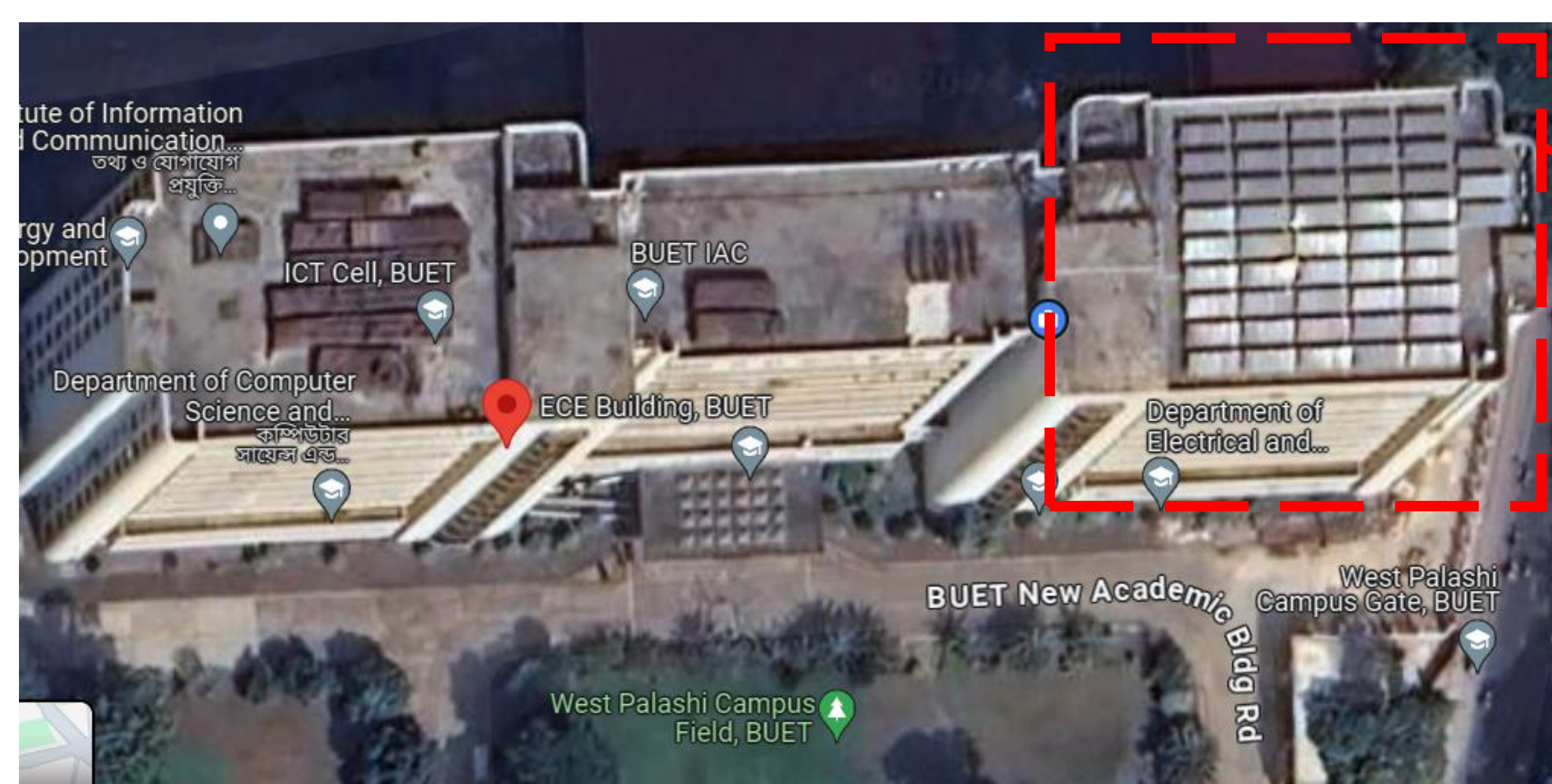
75 kW AC Rooftop PV System installed on the rooftop of ECE Building of BUET
